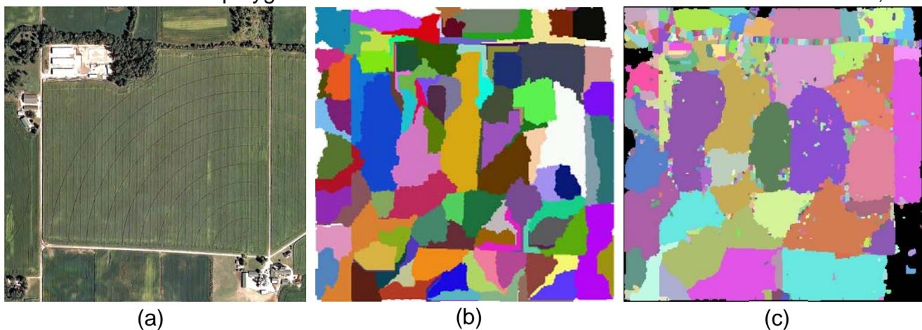
**Figure 7. Multi-Polygon Catchment Maps: a) reference image, b) those produced using a flow accumulation threshold assuming complete hydrologic connectivity, and c) those produced using our algorithm before all pits have been filled.**
