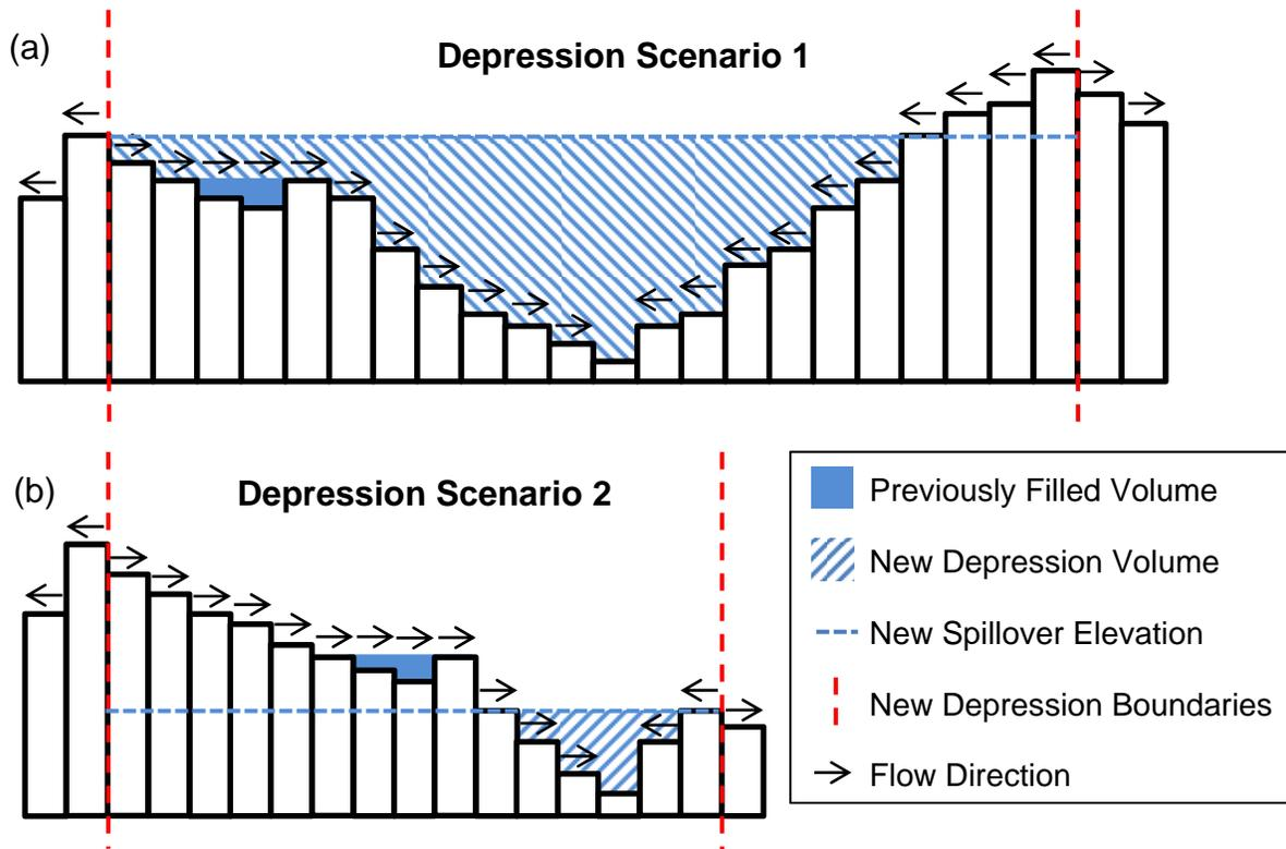
**Figure 3. Comparison of depression scenarios: (a) the total volume of the new depression is the sum of the differences between cell elevations and the new spillover elevation. (b) the previously filled depression retains water above the spillover elevation which necessitates recording any previously filled volumes as any two depressions merge.**
