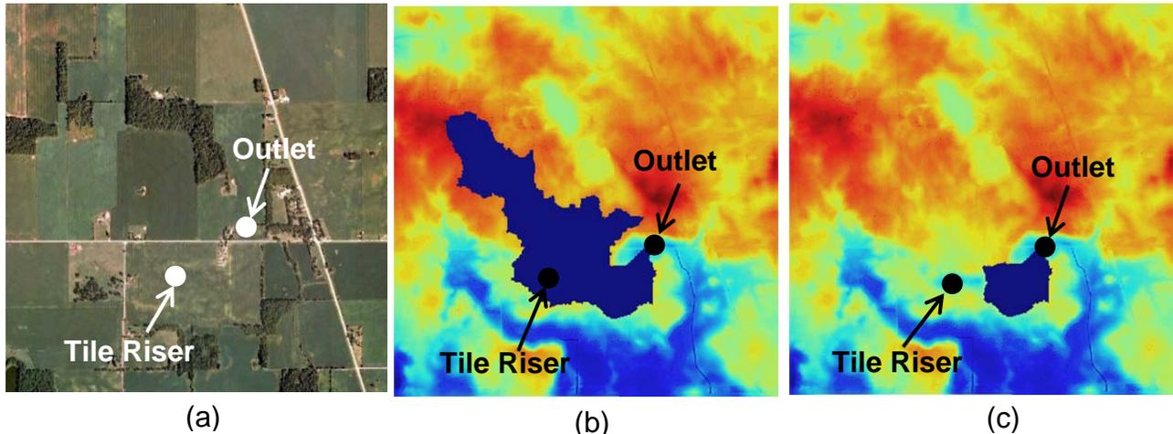
**Figure 6. Watersheds delineated (in dark blue) at the marked Outlet point: a) reference image, b) ignoring existing tile riser and c) including tile riser. Note that b) overestimates the contributing area whereas c) does not because drainage through the tile riser has prevented the natural depression from overflowing.**
