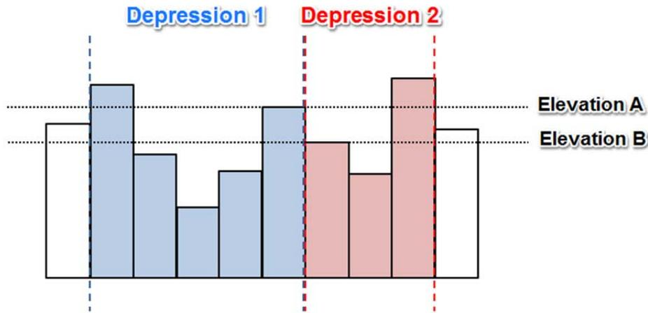
**Figure 4. Illustration of the need to look one cell beyond pit boundaries: the minimum elevation for Depression 2 is at Elevation B, but it will not overflow until filled to Elevation A.**
