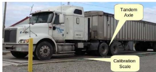
Figure 8: Experiment Vehicle Being Calibrated on a Scale
