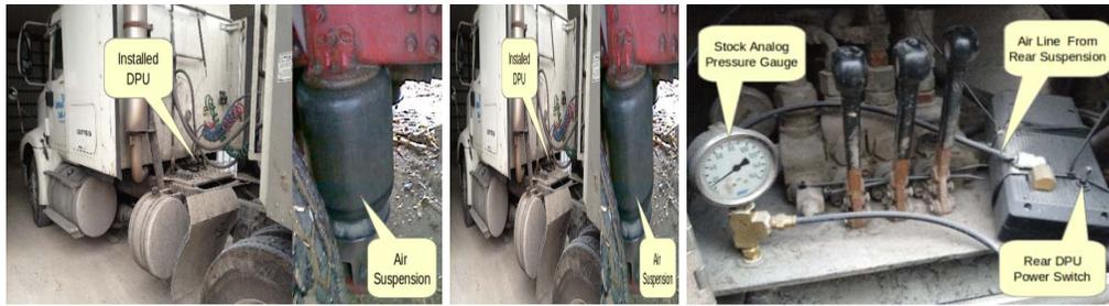
Figure 7: Photos of an Installed Weighing System.
