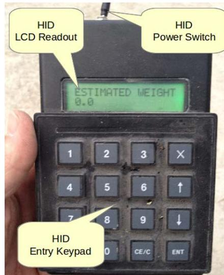
Figure 6: Human Interface Device for Displaying Weights and Identifying Calibration Data.
