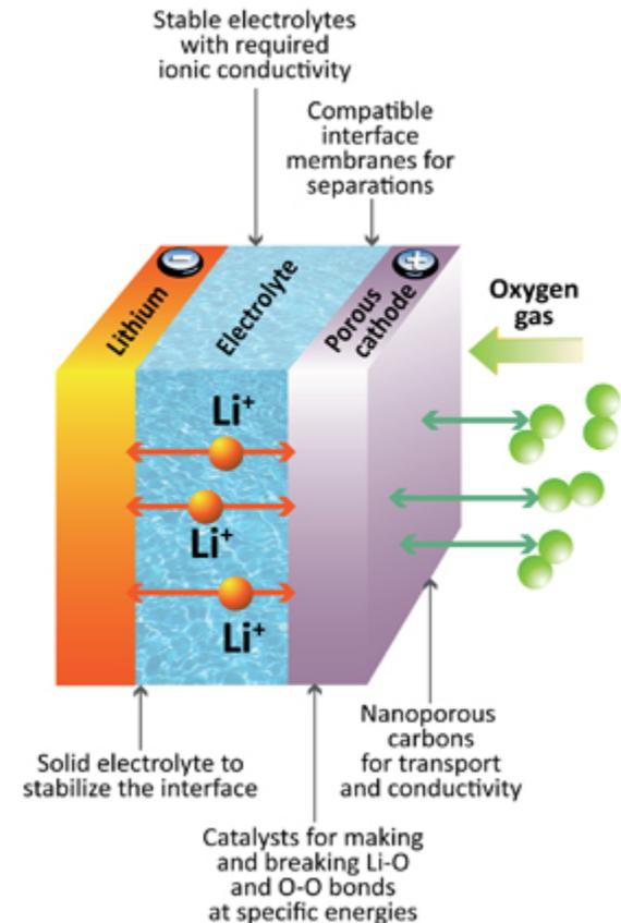
*Li-air batteries hold the promise of increasing the energy density of Li-ion batteries by as much as 10 fold.*
