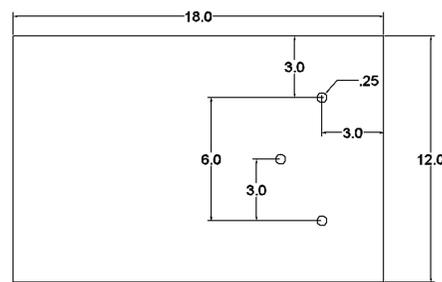
Fig 2. Shows the plate designed to be welded onto the bottom of the chassis dyno and secured down with concrete fasteners.
