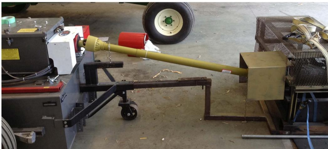
Fig 3. Shows the finished "Dual Dyno" system mounted to the floor and ready for initial testing.
