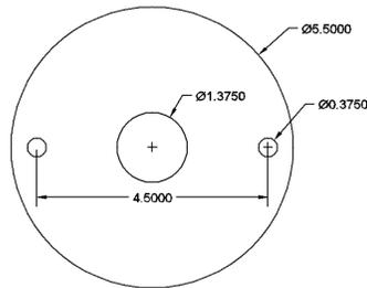
Fig 1. Shows the Plate design based on the stock PTO shaft mounting system on the PTO dyno which was fabricated and welded onto the new PTO Shaft.
