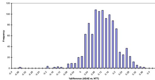
Histogram showing the difference between the ASAE fuel consumption equation and the regression equations created from the Nebraska Tractor Test data.
